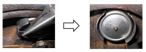
[Procedure 3] Remove air vent and spacer by hand.
