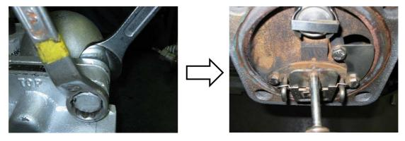
[Procedure 2] Remove the air vent holder with radio pliers.
