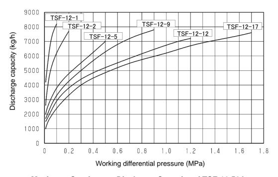
**Maximum Continuous Discharge Capacity of TSF-12 50A**
