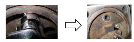
[Procedure 5] Remove the hexagon bolt on the upper side of the plate and the bolt on the inlet side of the float holder with spanner, ring wrench, etc (width across flat: 13mm). Then remove the plate.
