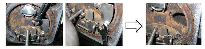
[Procedure 6] Remove the hexagon bolt on the outlet side of the float holder with spanner, ring wrench, etc (width across flat: 13mm). Then the float (P) and float holder can be removed. The valve is attached to the float (P).
