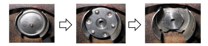
[Procedure 4] Remove the air vent valve seat with socket wrench (width across flat: 19 mm). Be careful as the valve seat has a gasket.
