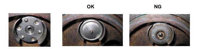
[Procedure 4] Air vent holder can be assembled by hand.
