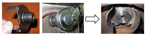
[Procedure 3] Put the spacer and attach the air vent in the air vent cover. Please pay attention to the direction of the air vent.
