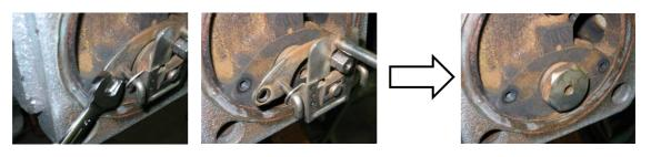
[Procedure 7] Remove the valve seat with socket wrench (width across flat: 39 mm).
