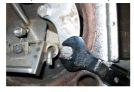
[Procedure 6] Put a new gasket on the cover and tighten the hexagon bolts and nuts fixing the body with 200 N·m torque using torque wrench (width across flat: 32 mm).
