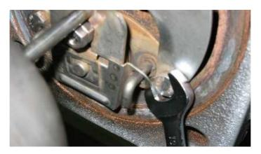
Then, align the spacer with the plate top hole and temporarily tighten the bolt.
